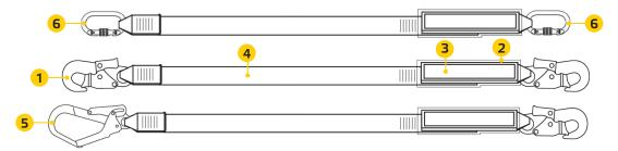
The Energy absorber is made of 32 mm wide webbing. The absorber is equipped with attachment loops on the endings which are integrated with a lanyard. The body of the absorber is protected by a special jacket made of a shrinkable, polyethylene tube. The lanyard can be made of 30 mm wide polyamide webbing. The endings of the lanyard are sewn making the attachment loops.
